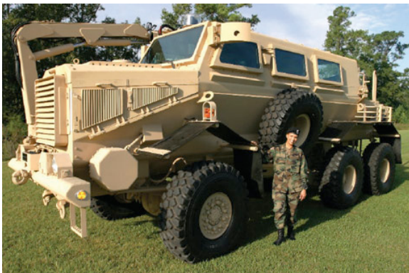
Three mine-protected, armored trucks in US service: from top to bottom, BAE Systems' four-by-four RG-31, Force Protection's four-by-four Cougar (also available in a six-by-six), and Force Protection's six-by-six Buffalo with its spork.
